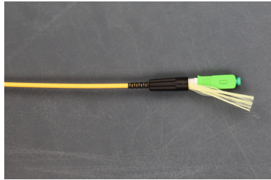
Step 16: Screw the tail boot 1-2 times. **Note: If it is difficult to screw the tail boot up, you may have to cut off excessive Kevlar.
