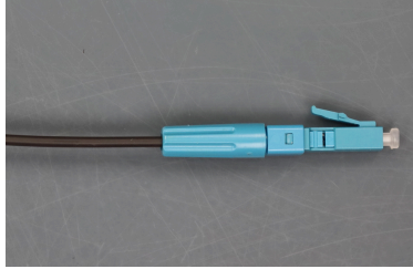
Step 13: Screw the tail boot up all the way to complete the assembly.
